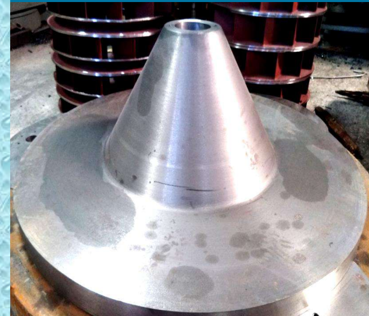
Casting Cone (Dia.1400mm, H-650mm)
