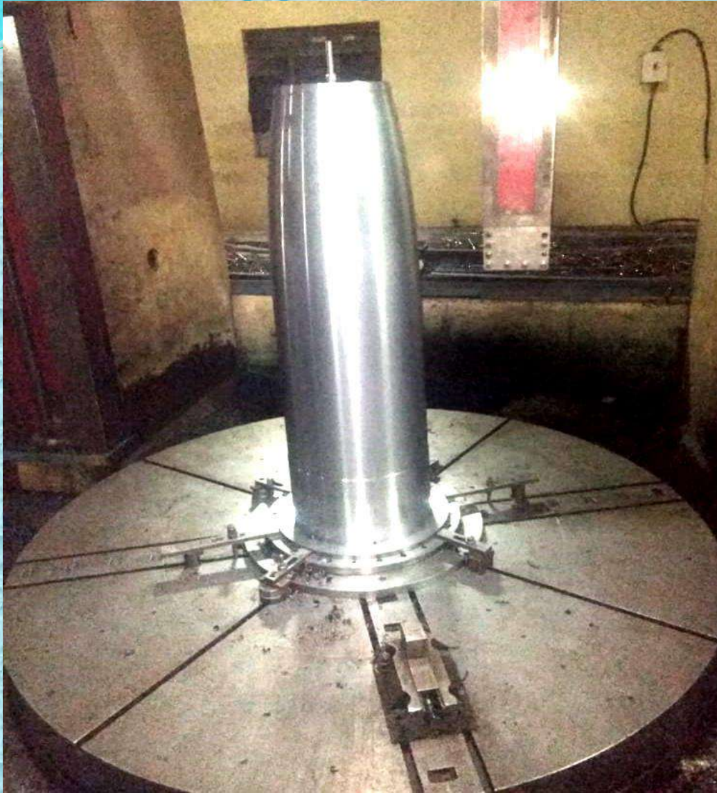
Machined Part(Dia.400mm, H-1.9m)
