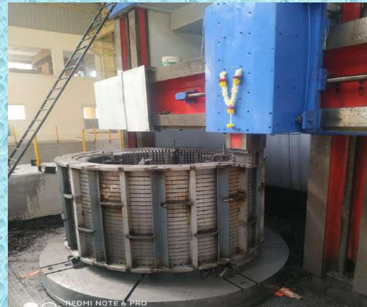
Stator Rotor Package(Dia.1.8m,H-1.4m)
