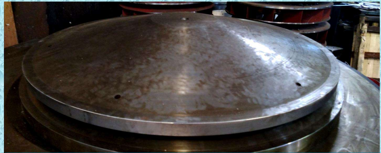
Inner Drum (Dia. 1m, T-125mm)
