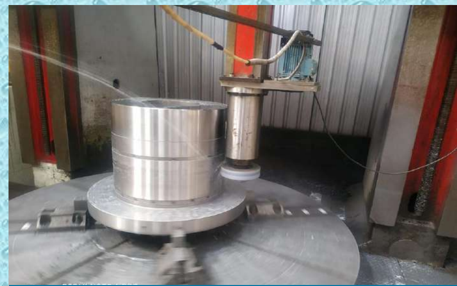
Runner Bearing(Dia.1.2m, H-800mm)
