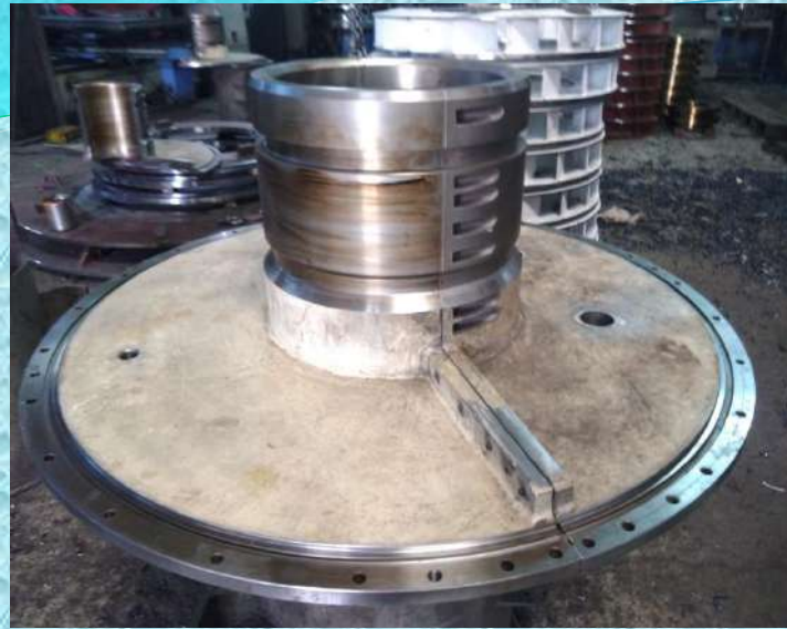
Stand Pipe(Dia.1.5m, H-0.6m)
