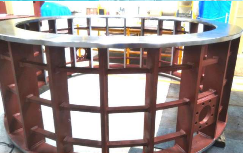
Stator Cage (Dia.3300mm, H-1200mm)
