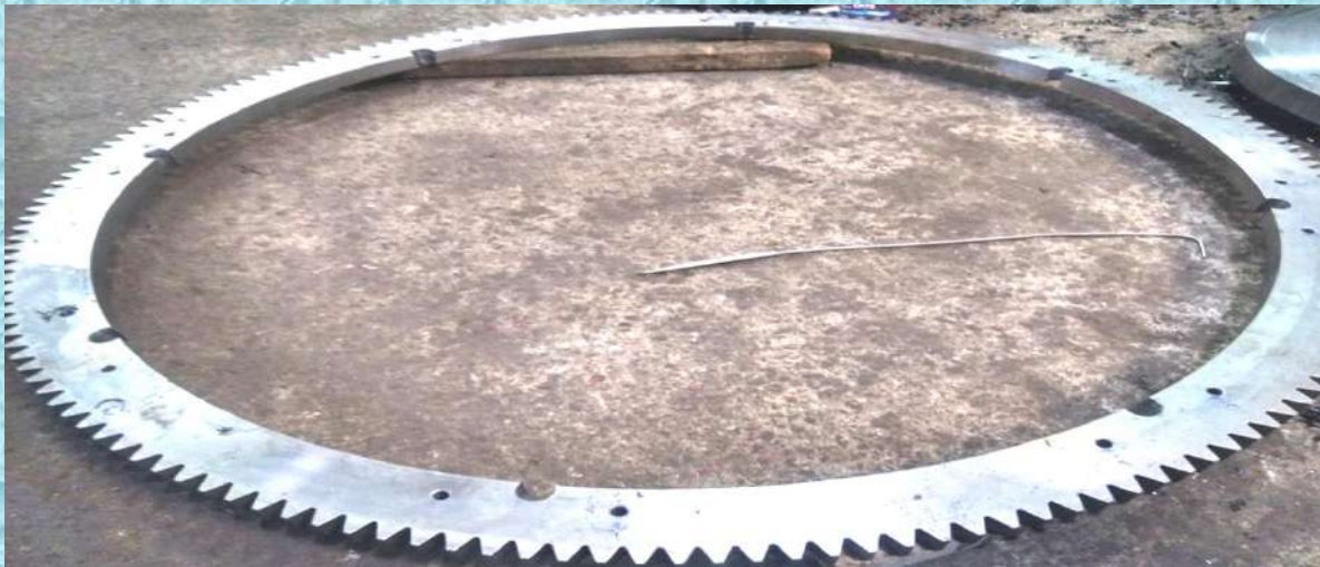
Gear- OD & Drilling Opt (Dia-2M)
