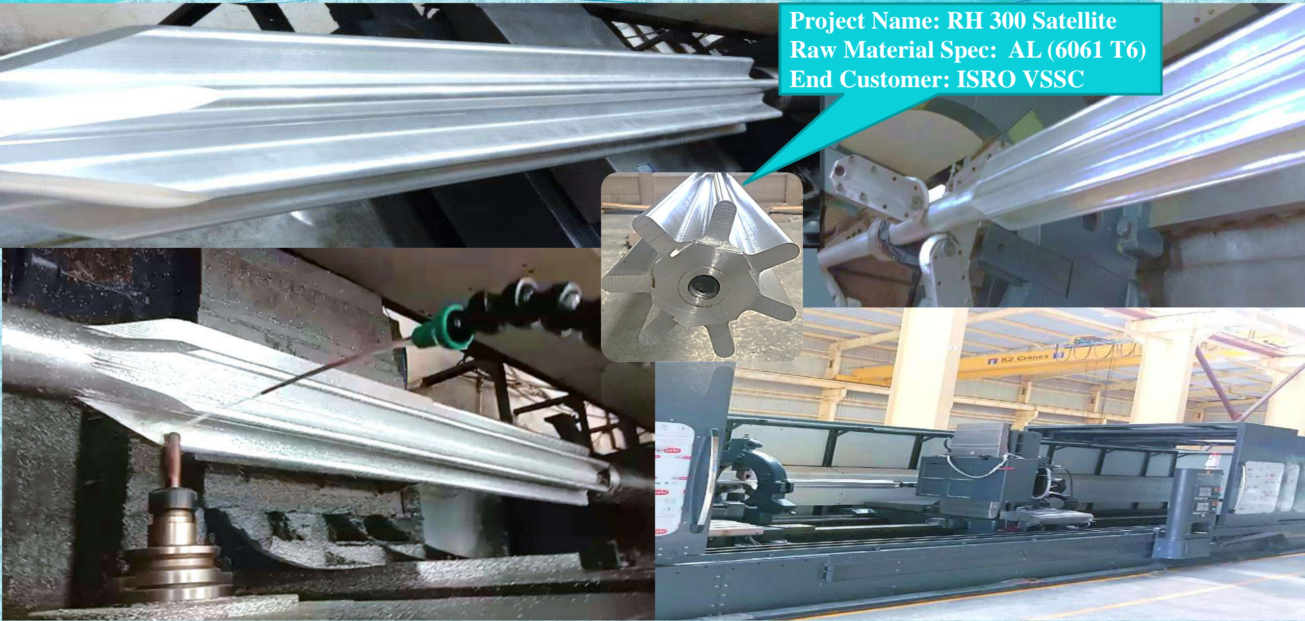
RH 300 Mandrel (Length-3400mm, Max Dia-165mm)
