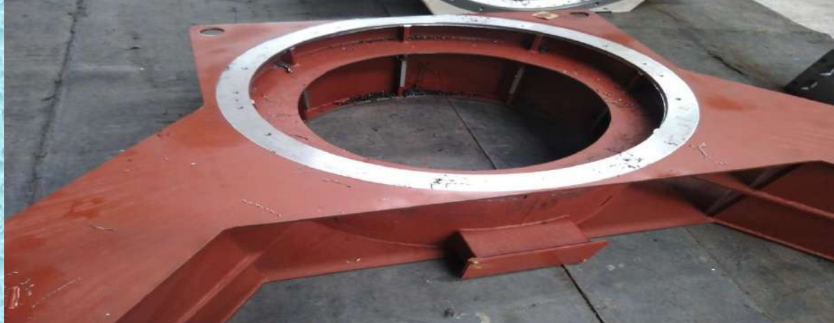
Exciter Frame(L-2.1m, W-1.5m, H-560mm)
