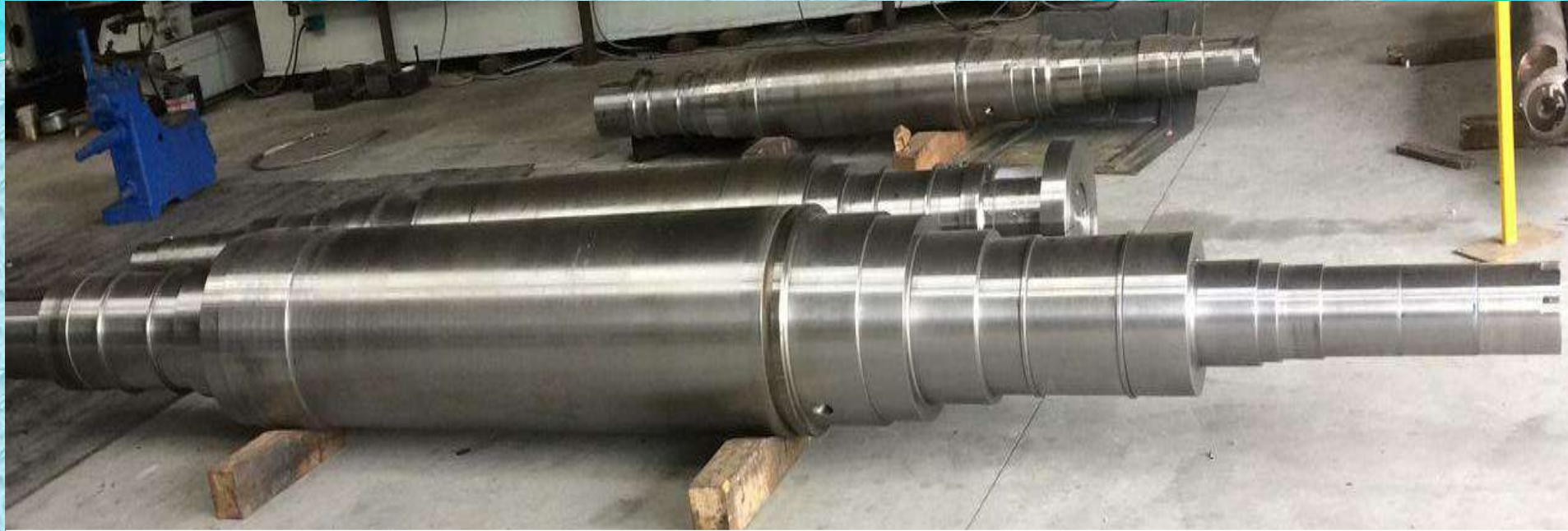
Shafts after Machining & Grinding
