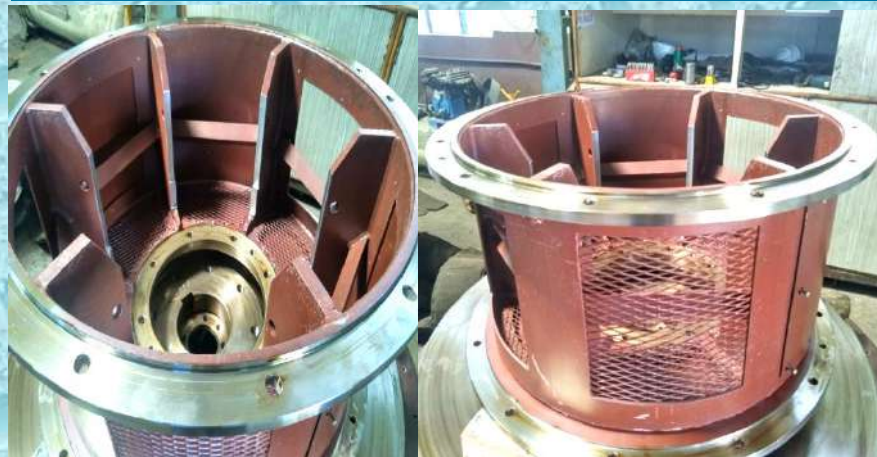
End Shield (Dia.800mm, H-800mm)
