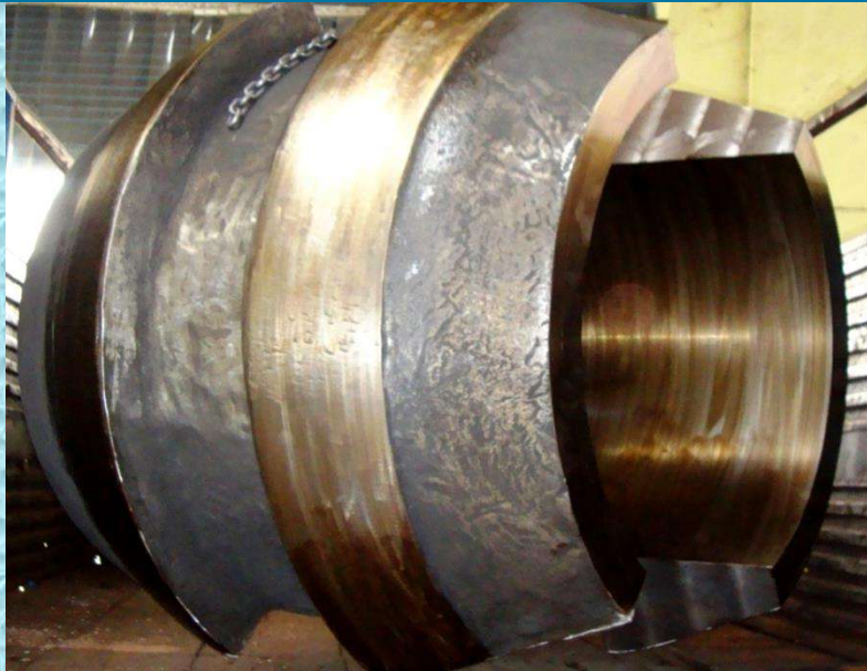
Housing Body (Dia.900mm, H-1.3m)
