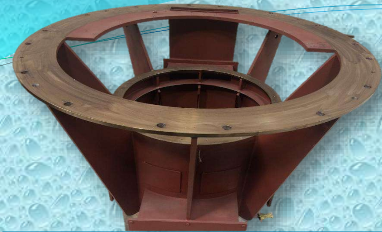
Exciter Stator Frame(Dia.2.1m,H-2m)
