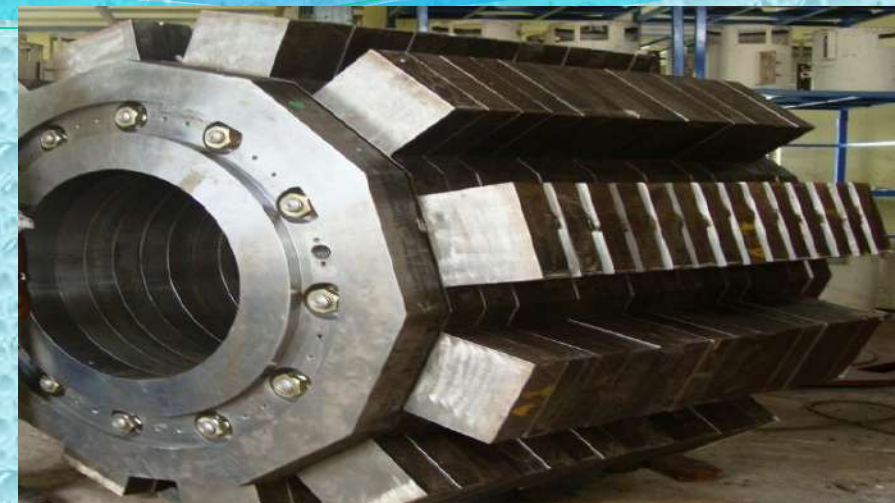
Rotor Hub(Dia.1.9m, H-1.7m)
